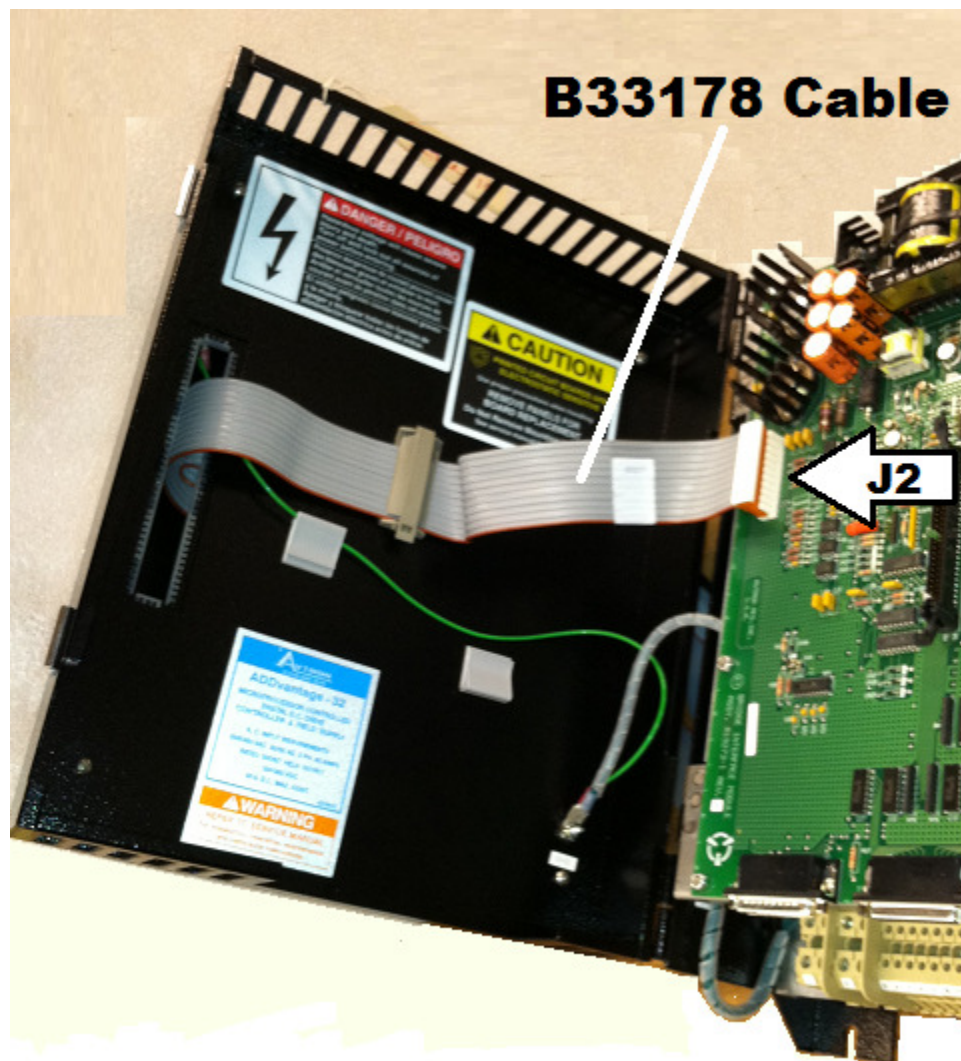
Figure 12-6. The B33178 ribbon cable plugs into connector J2 on the bridge interface board and routes across the drive cover.
