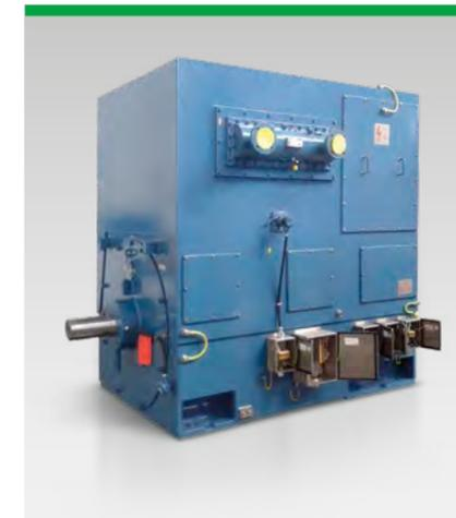
Organic Rank Cycle turbines are usually paired with 4-pole generators equipped with gearboxes. Desiring a more compact and efficient system, an OEM asked us to engineer a 2-pole generator that would not require a gearbox. We responded by designing a 2-pole synchronous generator that couples directly to the turbine to offer a more robust and efficient solution than the traditional configuration.
