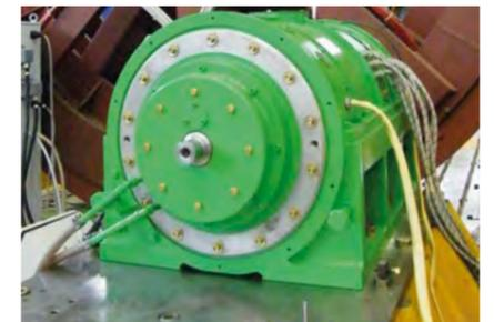
PM motor for high speed compressor
