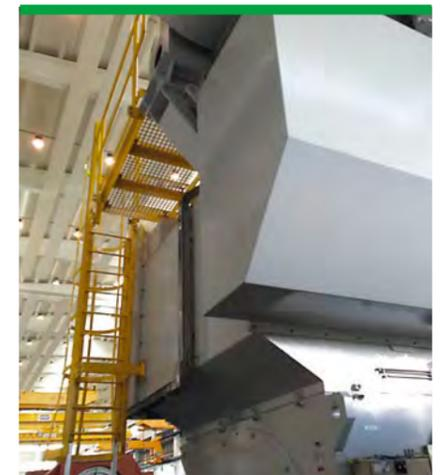
We supplied engineered-to-order synchronous motors for centrifugal compressors in a refinery. To facilitate field service operations and reduce inspection time, the customer asked us to design the motors with incorporated access stairs ensuring full compatibility with stringent safety standards.
