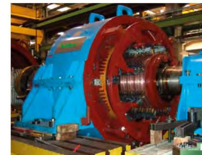
DC motor for cold rolling mill
