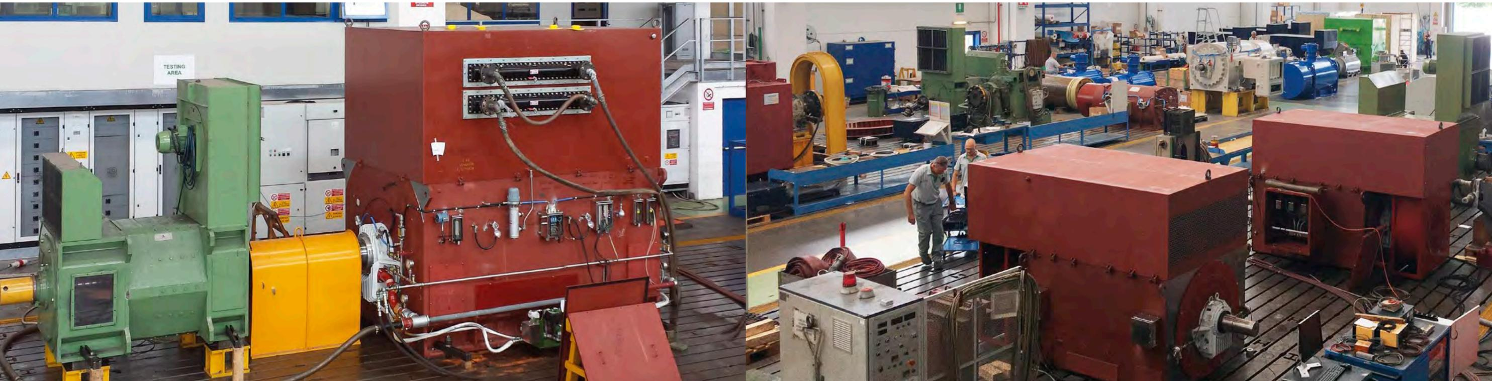
Our test room is one of the best equipped in Europe. Our internal test area measures 3600 mq with platforms that are fully equipped with MV AC and DC power supply and the necessary auxiliary circuits to run functional and performance tests on induction, synchronous and DC machines including full load testing capability up to 60 MW in back-to-back configuration. We also have an additional 1500 mq external test area for complete system tests.
