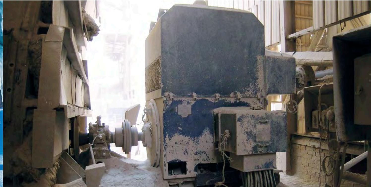
Induction motor for cement plant
